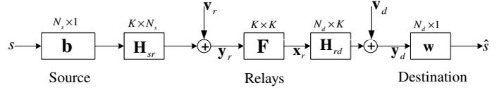
Fig. 2. Block diagram of the equivalent MIMO relay system.
