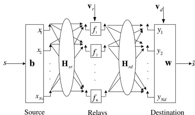
Fig. 1. Block diagram of a distributed MIMO relay communication system.
