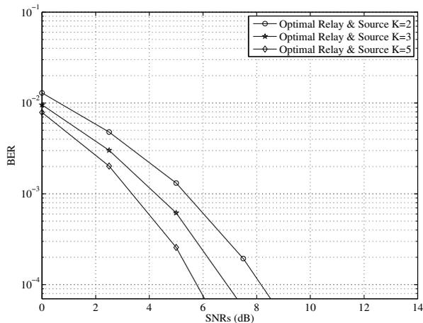
Fig. 4. Example 2. BER versus  $\text{SNR}_s$  with varying  $K$ .  $N_s = N_d = 5$ ,  $\text{SNR}_r = 20\text{dB}$ .
