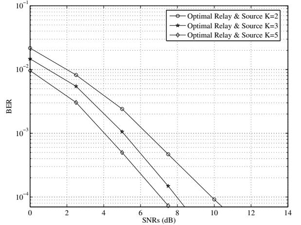
Fig. 3. Example 1. BER versus  $\text{SNR}_s$  with varying  $K$ .  $N_s = N_d = 3$ ,  $\text{SNR}_r = 20\text{dB}$ .
