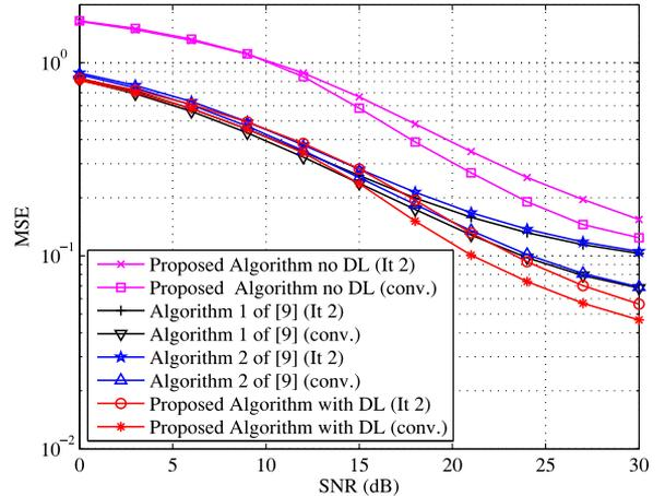
Fig. 2. MSE comparison of the proposed algorithm and the algorithms in [9].
