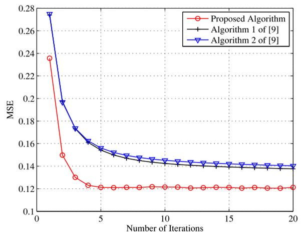
Fig. 4. MSE comparison of the proposed algorithm and the algorithms in [9] at different number of iterations.
