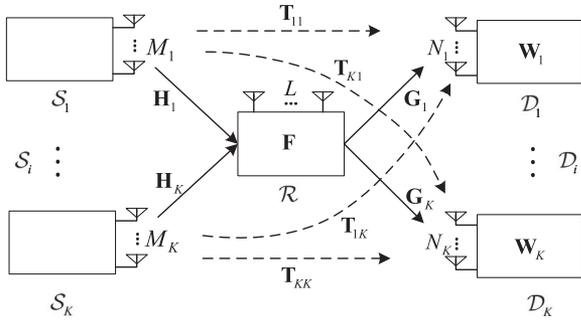
Fig. 1. Interference AF MIMO relay system with direct links.
