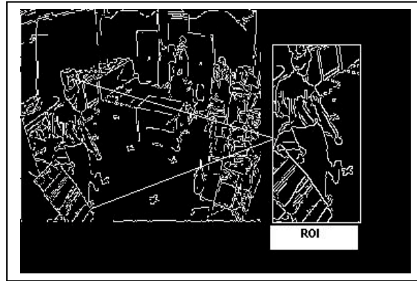
Figure 3. Canny Edge Detector and the region of interest (ROI)
