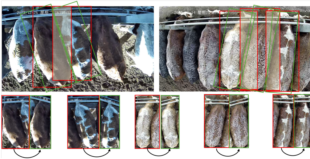
Figure 4. Comparison between axis-aligned and oriented object detection boxes: the red box represents the axis-aligned detection box and the green box denotes the oriented object detection box.
