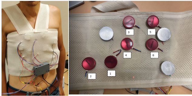
FIGURE 21. Prototype wearable vest holding six digital stethoscopes and one three-lead ECG sensor.
