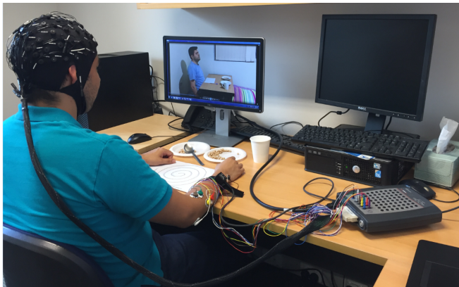
FIGURE 9. EEG sensors used as cap head for tremor recording.
