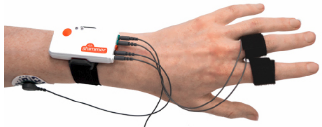
FIGURE 11. IMU sensors attached on a subject's wrist.
