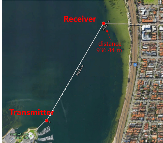
Fig. 3. Transmitter and receiver locations during the experiment.
